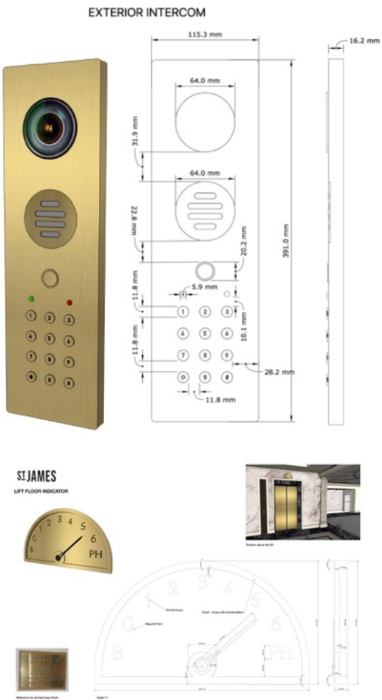
Lift & Intercom The lift and intercom were central to several sequences involving both babies and dogs. I designed the components for the prop makers and produced a full-scale 1:1 print of the lift interior and control panels so their exact positions could be worked out in advance for action and stunt planning.
