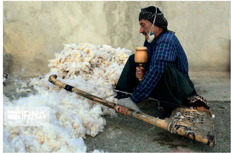
Above: Dhunai tool for traditional cotton spinning. Below: reference photo for Dhunai tool.
